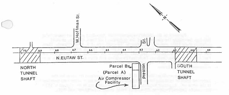
Appellant thus had to pipe compressed air from right of way Parcel "A" approximately 600 feet<sup>1</sup> to the North tunnel access shaft and 200 feet to the South tunnel access shaft. The routing of this piping network is the subject matter of this dispute.
